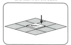
Make sure the LED panel is set properly inside the T bars of the ceiling.
