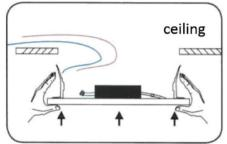
Wire the driver. With the tabs open, place the panel inside the ceiling.
