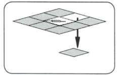
(5) Remove a ceiling plate from the close to the LED panel.
