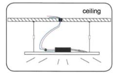
6 Connect the driver to the electrical network.
