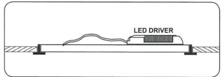
(7) Replace the plasterboard to complete the installation.
