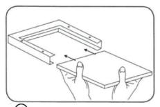
Attach the LED panel to the frame by sliding it.
