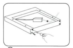
6 Finish the electrical installation and screw the frame.
