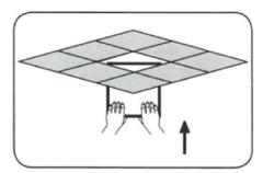
3 Place the LED panel on the ceiling grid.
