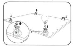
2 Fasten the tabs to the same positions as the removed screws by screwing in the center.
