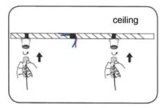
4 Screw the cable to the ceiling mount.
