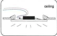
Grip loops gently until the panel fixes on the ceiling, completing the installation.
