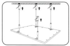
5 Attach the LED panel to the ceiling, and make final adjustments to the desired height.
