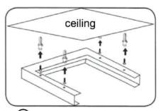
Screw the frame into the ceiling
